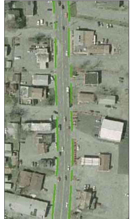
Above: Aerial view of the Ulster Avenue Corridor north of the City of Kingston. The areas in green show where landscaping islands or curb cuts could be placed to help define driveways in order to better control access into and out of development sites. Many existing sites within this corridor do not have curb cuts to control access. The corridor is not pedestrian friendly, but the provision of sidewalks and controlled access to commercial sites would make the corridor more pedestrian friendly.
